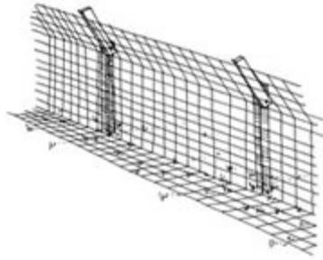
**Figure 6.** Fence extensions are required to keep coyotes from jumping over a 5-foot fence. Angle the top of a woven-wire fence out about 15 inches and completely around the fence. An effective fence extends below the surface, or has a wire apron in front of it to prevent digging.
