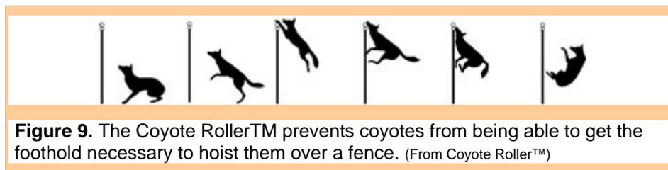
Alternatively, install a commercial device, such as the Coyote Roller™, to prevent coyotes from being able to get the foothold necessary to hoist them over a fence (Fig. 9). (See “[Internet Resources](#)” for additional information.)
