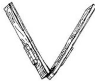
**Figure 5.** Construct a clapper by hinging together two, 24-inch 2 x 4s. Smack the two sides together.
