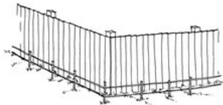
**Figure 8.** Two electrified wires, 8 and 15 inches above ground and offset from an existing wood fence by 12 inches will prevent coyotes from accessing the fence. A single strand may be sufficient, but two electrified wires will provide added insurance.
